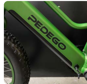
Battery Fully Installed
