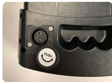
52v Charging Port
