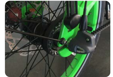
Internal Nexus 3 Speed Hub and Bell Crank
