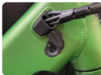
48v Charging Port
